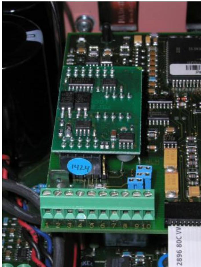
Jumpers in picture configured for the last inverter in the RS485 network
